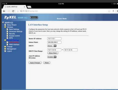
(Lan interface set-up including DHCP server configuration)
